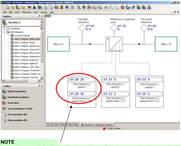
It should be noted that if the drive is set for an Open Loop mode, these registers will be in Hz vs RPM. So something like 0.5 - 1Hz may be a reasonable value in this mode.
