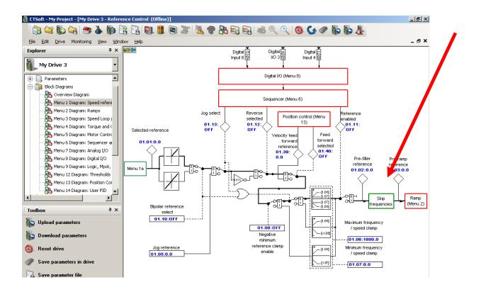
What I would suggest is to simply place a low value in the Skip Speed and Skip Band. Select a value that can be made as large as possible thus rejecting or blocking any low input signal below a certain valid value. Setting the same value in each register will provide pure digital symmetrical blocking band around 0 and will not disturb bi-directional operation if required.
